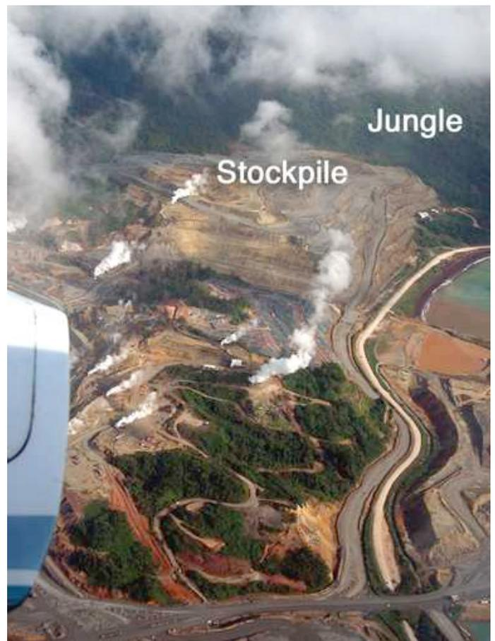
Figure 4. Persistent cloud cover and steam plumes rising from geothermal pressure relief wells posed a problem for LiDAR data collection. The large barren earthwork in the middle ground is an ore stockpile, and the dark area in the distance is dense jungle cover.
