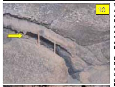
To monitor movement cave rock, informal wooden pegs or "tattle tales" were set upright within open joints. Pegs would have fallen if disturbed by rock mass movement (Figure 10), but none fell.
